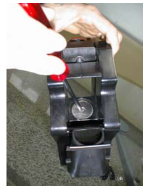
Dismount the inferior filter and clean it with hot water removing all coffee powder.
