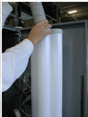
Fill in with appropriate cups all the columns of the tower.
