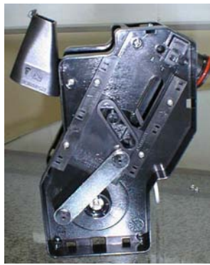
Turn the group in the position of ejection waste grounds and overturn the slide of coffee
